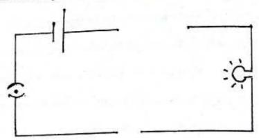
ii. Mark the polarity of each component and show the direction of current (4)
